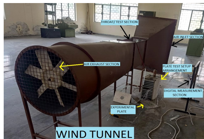
Fig. 1: Wind Tunnel Test Rig.
